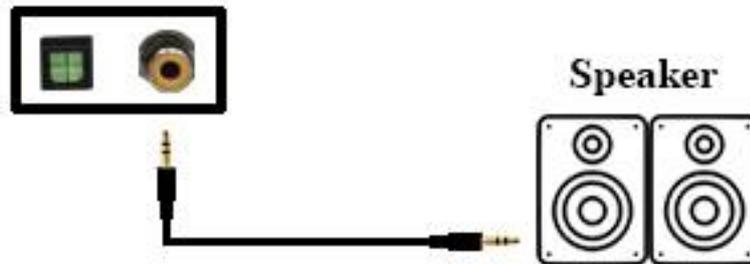
Figure 6-5: Audio Output Connection
