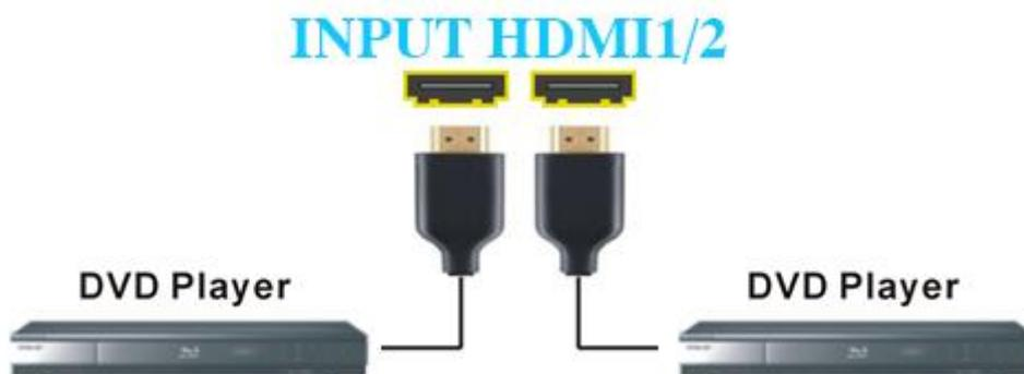
Figure 6-2: Input Connection-HDMI
