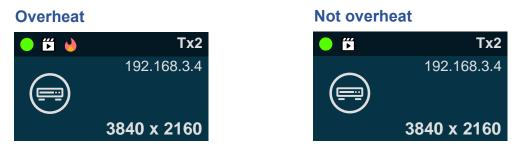
Figure 7-24 Device card overheat status
