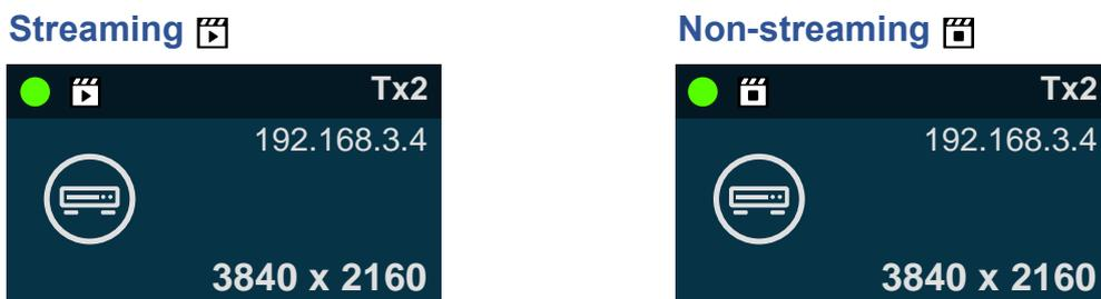
Figure 7-23 Device card streaming status
