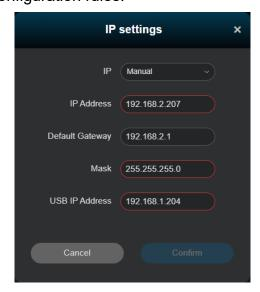
Figure 7-102 Edit device IP window with invalid values
