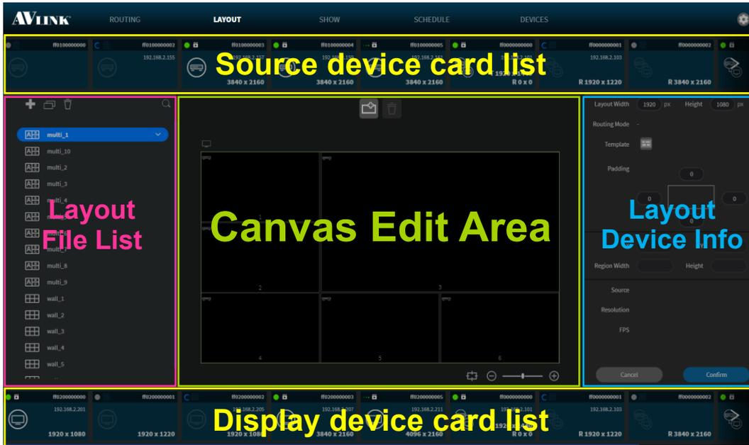
Figure 7-13 LAYOUT configuration
