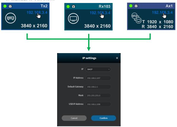
Figure 7-101 Edit device IP window
